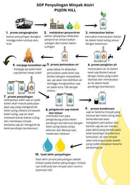
Gambar 3. Standard Operational Procedure Penyulingan Minyak Atsiri
